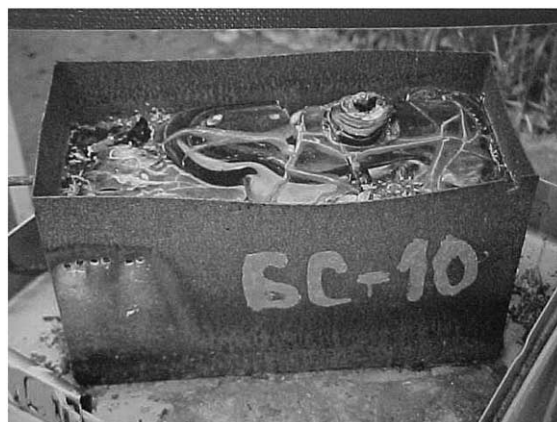
Fig. 1. Block of waste glass Bs-10 in a carbon steel container placed on the stainless steel tray at the open testing site.
